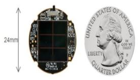
Fig. 3 Tiny Solar BLE temperature and humidity sensor [18].
