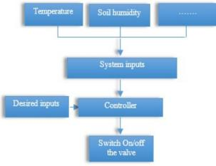
Fig. 6 Block diagram of the irrigation controller.
