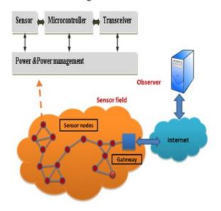
Fig. 2 Wireless sensor network architecture.
