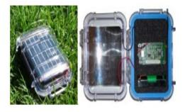
Fig. 5 Heliomote solar harvesting sensor node [20]
